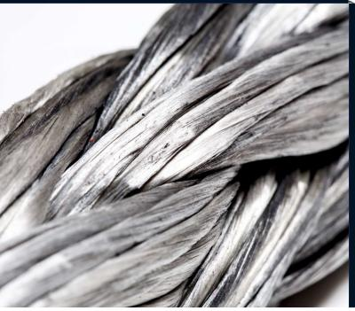
The HMPE ropes go through a special heat and UV resistance treatment. They have an extremely low friction coefficient and highly reduce an operation costs. Additionally, they offer much safer handling solution compared to a standard steel wire ropes.
