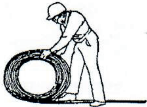
Figure no. 5: rope uncoiling - rolling out over the ground
