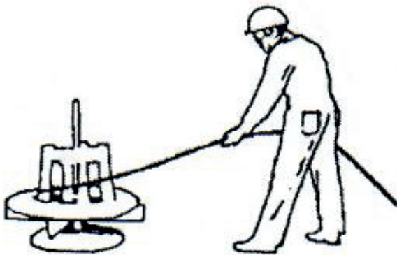
Figure no. 4: rope uncoiling - turntable
