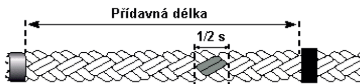
Figure no. 6: Marking the length of splice
