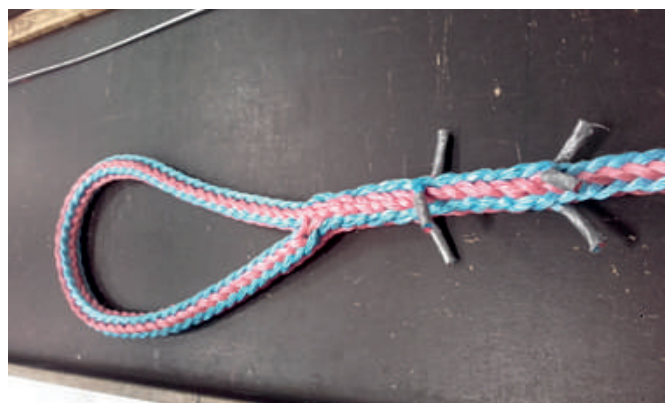
Figure no. 25 b): Finished splice
