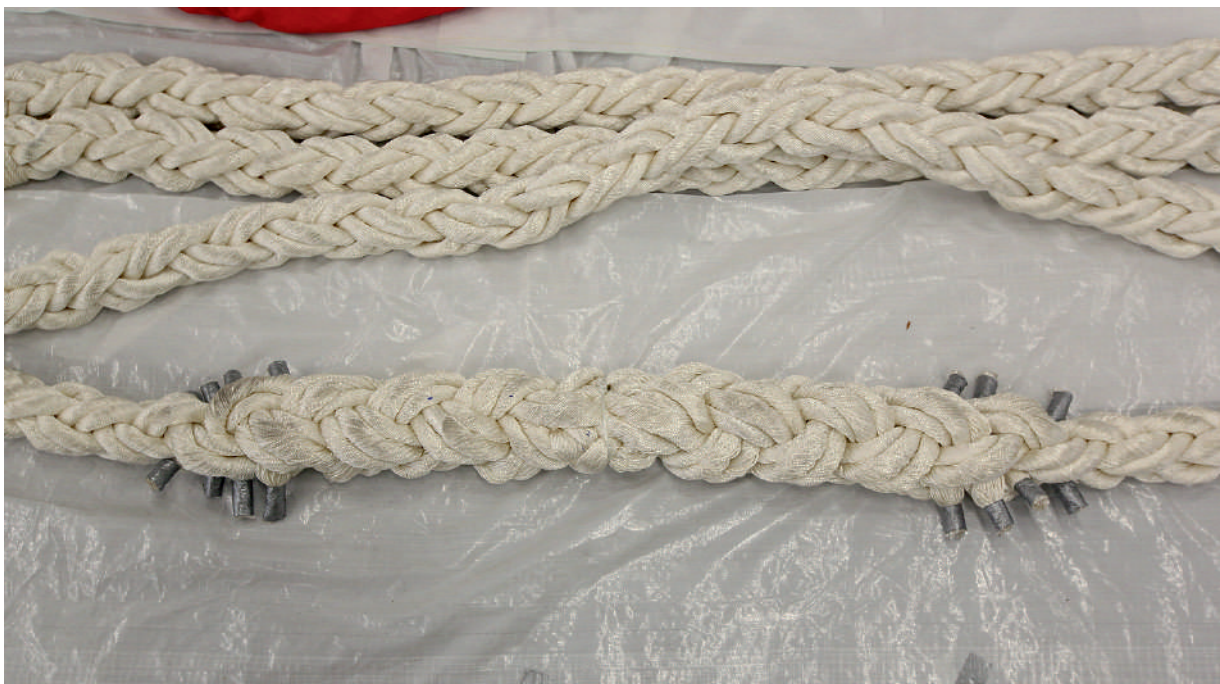
Figure no. 18: Finished splice
