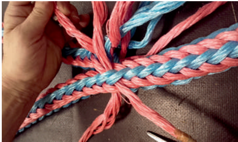
Figure no. 23 b): Tucking the "S" strands
