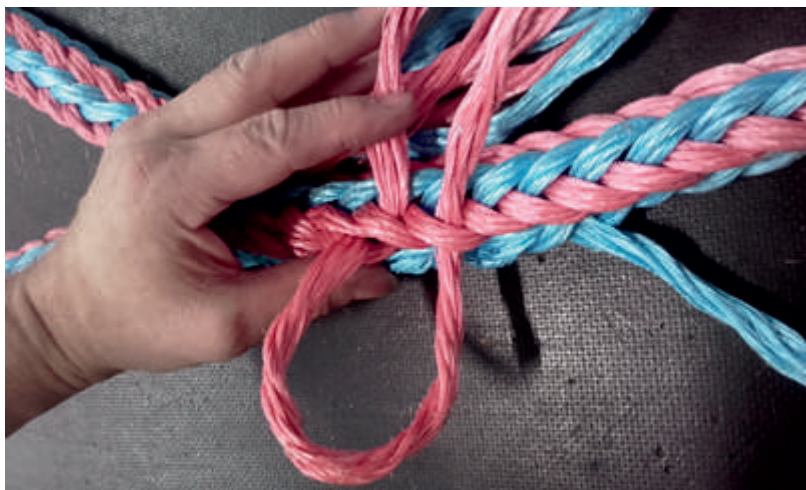
Figure no. 23 c): Tucking the "S" strands
