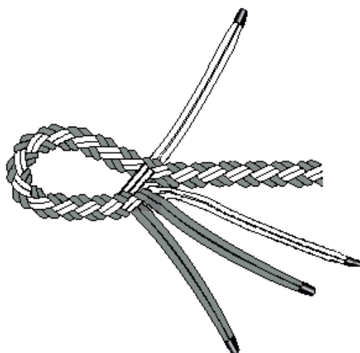
Figure no. 7: Finishing the splice
