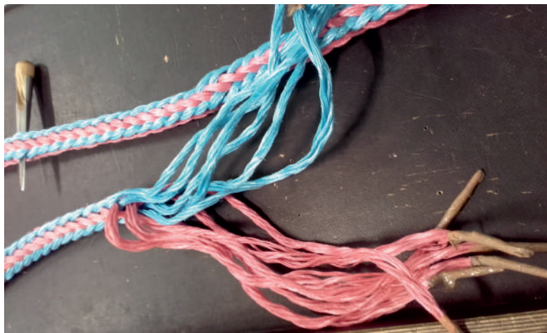
Figure no. 19: Marking the length of splice and unbraiding of individual strands
