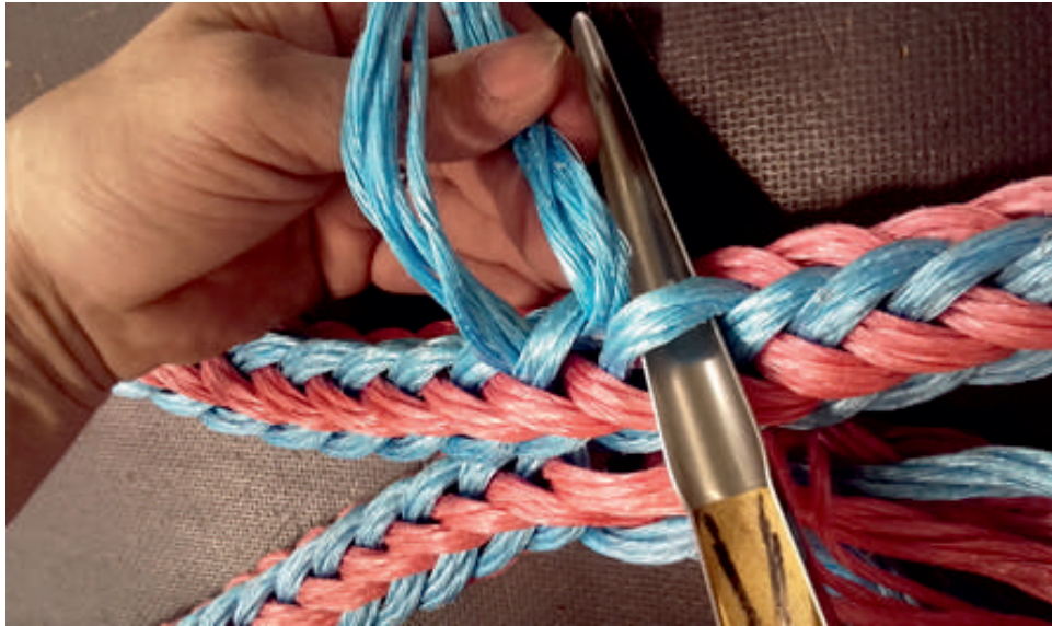
Figure no. 21: Lacing both "Z" strands
