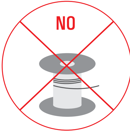
Figure no. 4: not recommended spinning of the reel
