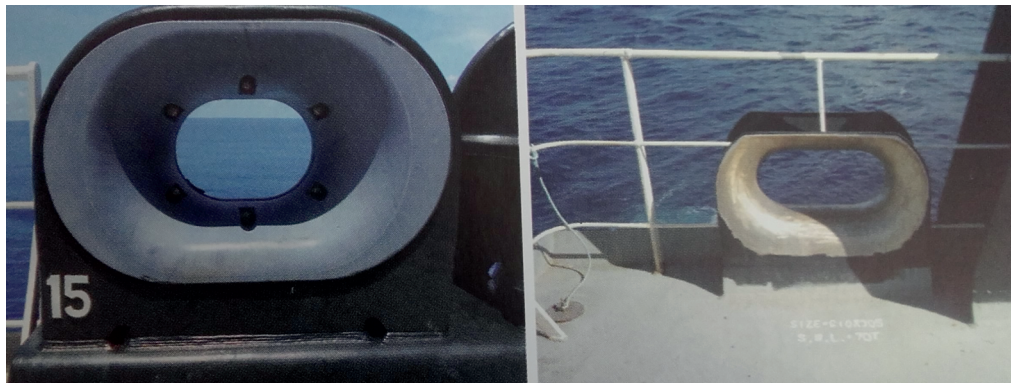
Figure no. 2: Polymer and stainless steel insert in fairleads
