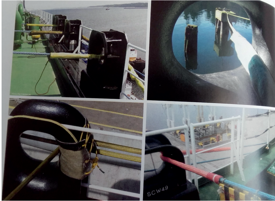
Figure no. 1: Chafe protection on lines and in fairleads
