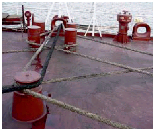
Figure no. 4: Incorrect line routing
