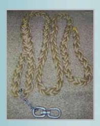
Ragger Rope with a double swivel and fastening hardware is recomended by all Waste Paper Pulper Producers and all Ragger Manufacturers.
