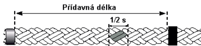
Figure no. 6: Marking the length of splice
