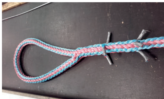
Figure no. 25 b): Finished splice
