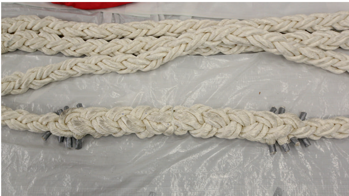
Figure no. 18: Finished splice
