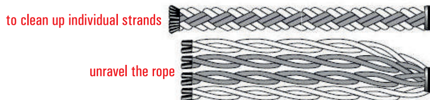
Figure no. 14: 8-strand braided ropes (end-to-end) - step 3
