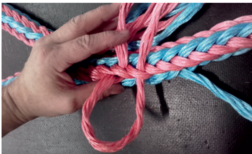
Figure no. 23 c): Tucking the "S" strands
