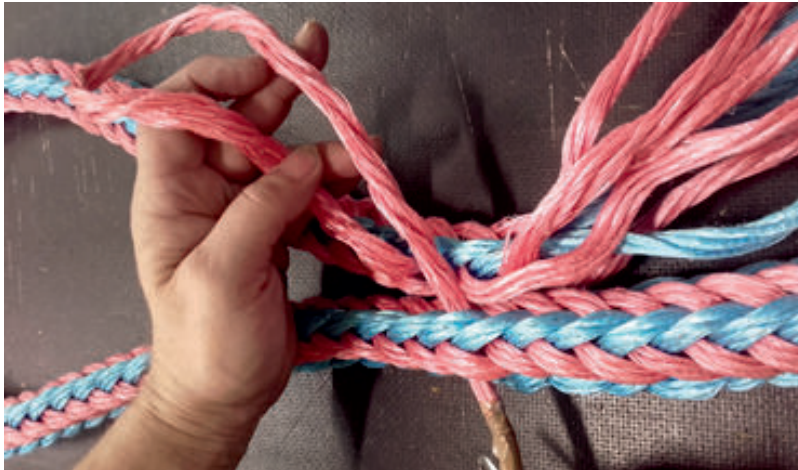
Figure no. 23 a): Tucking the "S" strands
