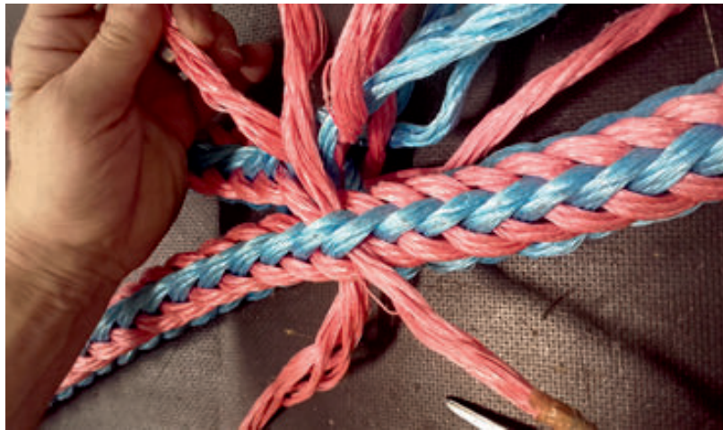
Figure no. 23 b): Tucking the "S" strands
