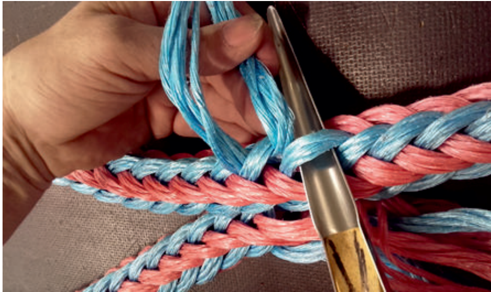
Figure no. 21: Lacing both "Z" strands
