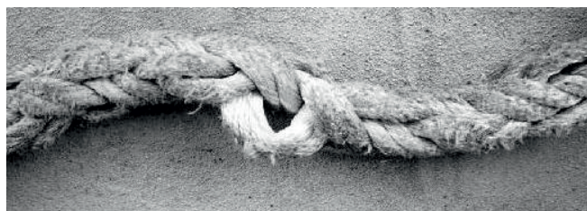
Figure no. 10: Localized external abrasion 2
