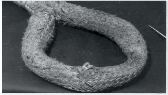
Figure no. 11 b): damage of splicing - wear in double braid eye splice
