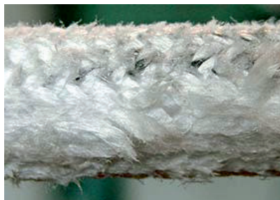
Figure no. 15: Melting of fibers
