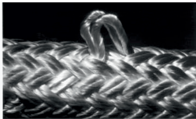
Figure no. 9: Localized external abrasion 1
