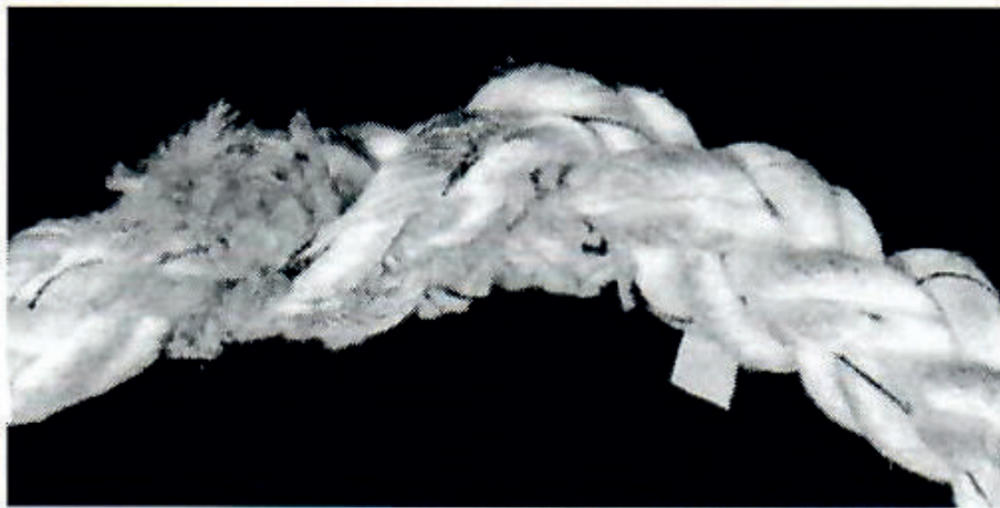
Figure no. 8: Localized external abrasion
