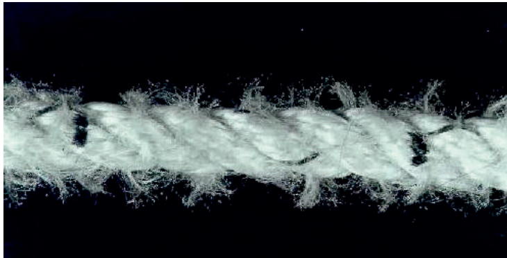
Figure no. 14: UV degradation of PP rope
