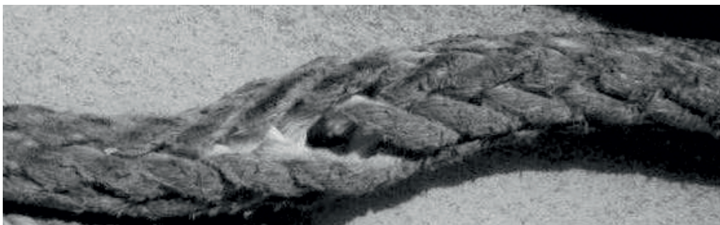
Figure no. 4: Inter-strand abrasion (exposed internal area reveals wear at strand internal contact points)
