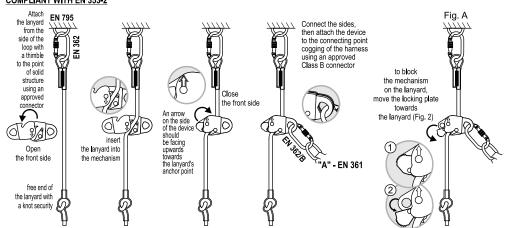
The CATCHER device used for arresting the fall should be attached only to the cogging point of the harness compliant with EN 361. The cooging point must be marked with letter 'A' Fig. B
