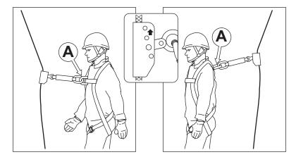
**ATTENTION**: Every time before using the equipment protecting against falls from height that employs the LANOSTOP one needs to check if all the components are properly interconnected to one another and cooperate smoothly, as well as if they are compliant with compulsory standards:
