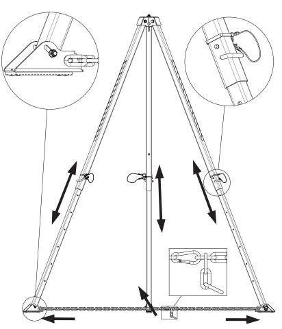
MAXIMUM LOAD TRANSMITTED FROM THE TM 9 TO THE STRUCTURE / LOADING DIRECTION Surface, where the TM 9 safety tripod was placed on must support the max. device load of 12 kN. Loading direction: perpendicular to the surface on which the TM 9 safety tripod is placed.
